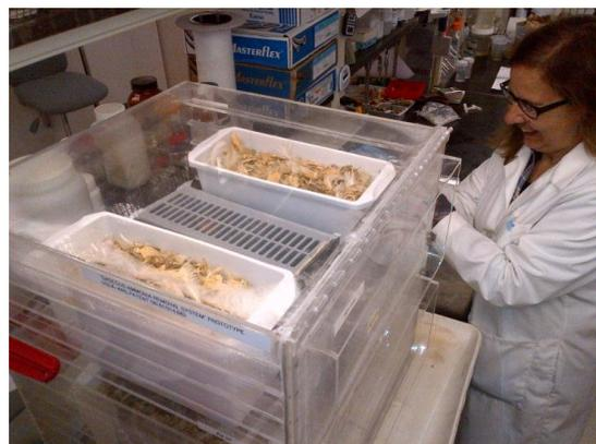
**Figure 2.** Prototype ammonia recovery system using gas-permeable modules (duplicate tests). One chamber circulated acid solution and the other circulated just water.
