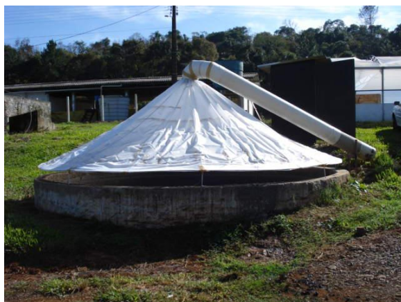
Figure 1. Dynamic chamber installed above the manure storage pit to continuous assessment of the emission of CH 4 , CO 2 and N 2 O.
